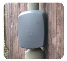
One tool used to monitor usage of the routes is a number of beambreak electronic 'pedestrian counters' which are installed around the routes. For the latter two routes, Bicester West and Bicester North-East, these were installed a couple of months ahead of the line being in place, to allow us to have an idea of the background pedestrian traffic along the routes, and to be able to measure the increase once the route had been marked out.
